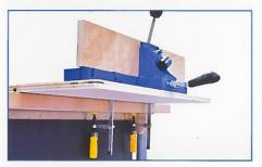
Bench mounting tools is quick and easy. Simply cut a couple of dovetail slots in a scrap of ply for each benchtop tool and swap tools in seconds.
