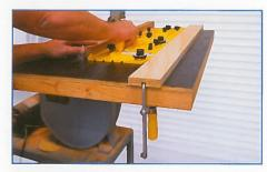
Custom fences, like this one on a bandsaw auxiliary table, can be made to order in minutes. This makes the most of your shop machines and time.
