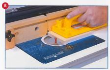
Create a dovetail groove in your workpiece using a router with the 1/2" diameter, 14° dovetail router bit.
