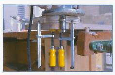
Templates for routing can be sized as needed. No exposed clamp heads to get in the way of your router base.
